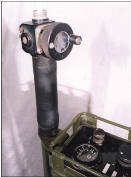
Fig. 3: The LSP-30 tuning section, rotating the tuning raises or lowers a plastic-connecting plunger (see text).
