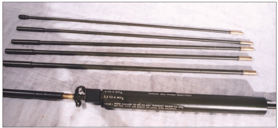
Fig. 9: The PRC-74 loading coil and 5-section whip antenna.
