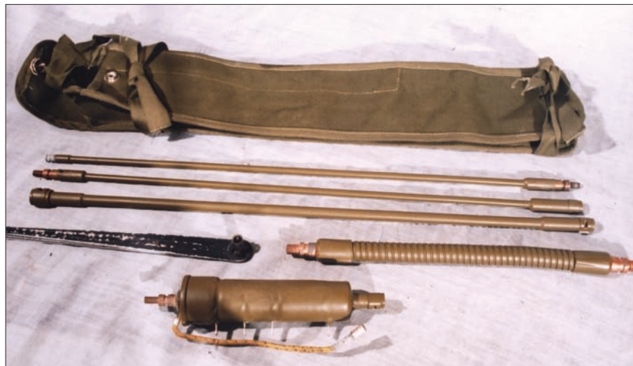
Fig. 7: The Chinese whip with tapped loading coil, flexible section and 4-leaf 'petal' type capacity hat (see text).
